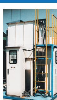
外圧浸漬式中空糸膜装置 External pressure immersion type hollow-fiber membrane equipment
