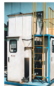
外圧浸漬式中空糸膜装置 External pressure immersion type hollow-fiber membrane equipment
